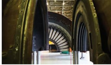
Far left: **The Darlington turbine hall. For the first time all turbine blades and rotors were removed and reinstalled to ensure continued operation for another 30 years**
