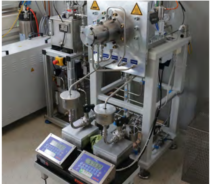
New fueling machine ram seals were developed through a COG joint project that tested for long-lasting performance before they were put into service at two COG member plants.
