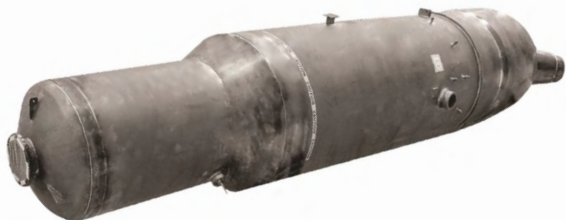
A 145-tonne steam generator. Image: Bruce Power
